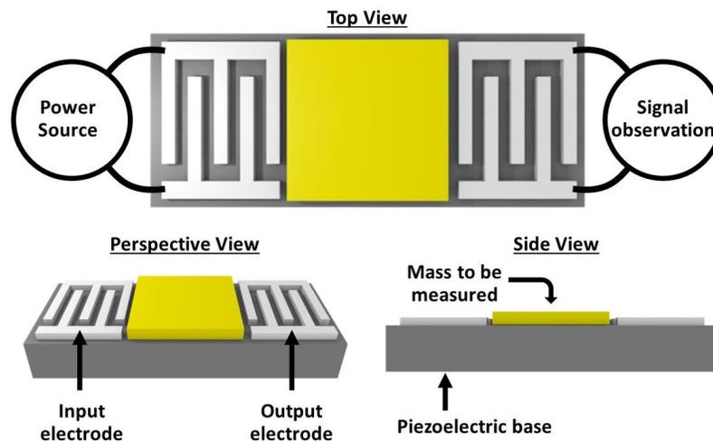
In these sensors, a wave is generated at the input electrode, which travels through a sensor material (yellow) and arrives at the output electrode. Depending on the mass of the sensor material, the wave will travel more quickly or more slowly. This traveling wave phenomenon can be modeled by the following partial differential equations:
